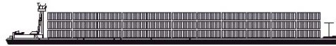
Container ship Jowi-class length 135 m. width 17 m. depth 3 m. load capacity 470 teu
